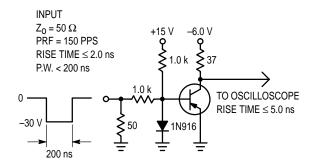
Figure 2. Storage and Fall Time Test Circuit
